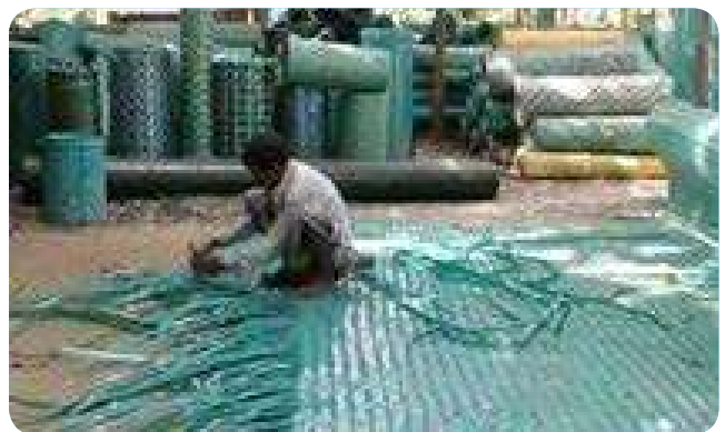
Plastic mats prepared from waste plastic strapping
