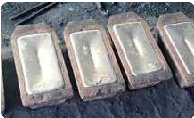
Aluminium extracted from waste foil
